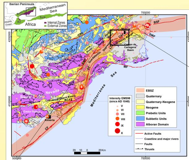
The Carrascoy Fault (CAF) is located in the Internal Zones of the Betic Cordillera (Southern Spain). It is one of the main faults forming the Eastern Betic Shear Zone (EBSZ), a major structure accommodating the convergence between Nubian and Eurasian plates at the westernmost part of the Mediterranean Sea (Larouzière De et al., 1988; Silva et al., 1993).
