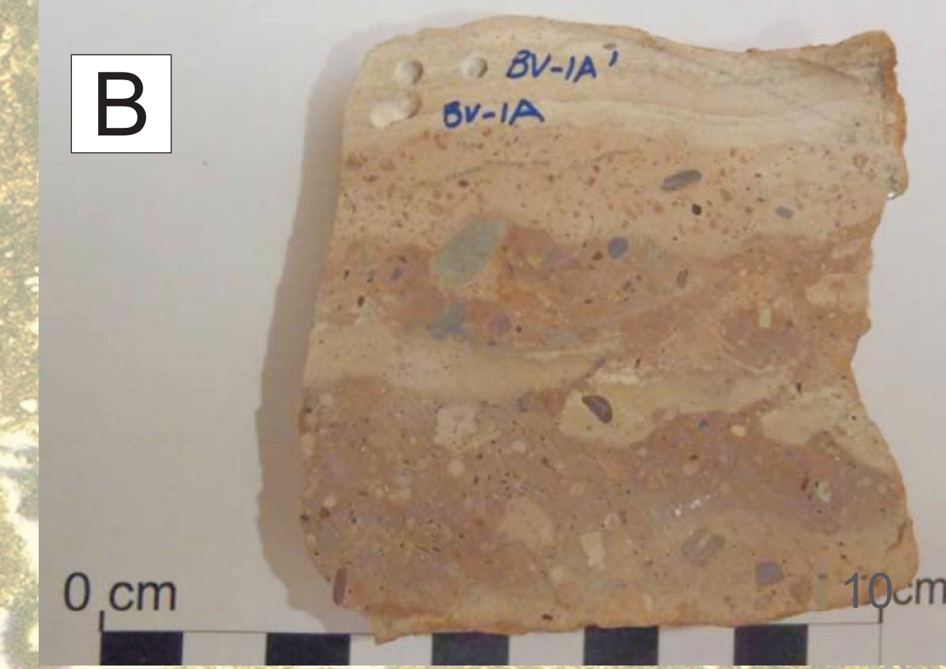
Figure 5: B) Hand specimen of the laminar calcrete and points sampled for U/Th analysis.
