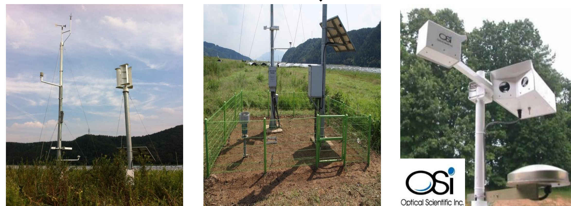
(a) N11 Point of Gangjeong–Goryeong Weir in Nakdong River (b) Visibility measurement: OWI-430 DSP-WIVIS
