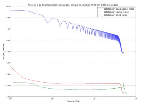
As those embedded ADCs are only 12bits and lower range dynamic than the commercial seismological dataloggers, it makes them unusable for study of seismological noise. May be in a
