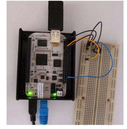
Just for fun, we tried to evaluate if those embedded ADCs could digitize seismological signal. We calculated its eletronic noise by using a method described by R. Sleeman et al. (C) and
