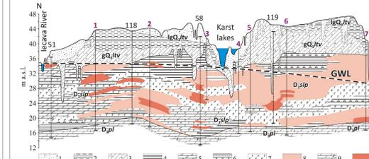
Fig. 3. Geological section of the study area along the line of sampled wells (Nos. 1; 3; 4; 7), the length of the section is 2.6 km (Tracevska et al. 1986)
