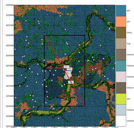
Fig. 7. Model setup: black frame – area of interest; green dots – assigned tophead; numbers – calibration wells; grey dots – wells for geometry building; red line – cross section (see Fig. 9.)
