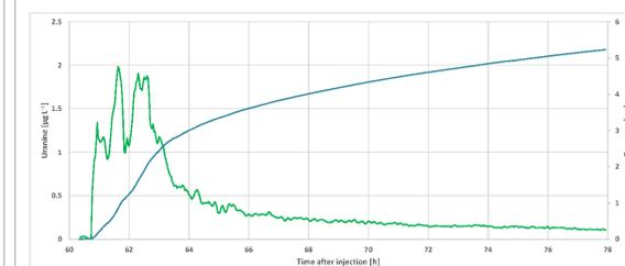
Fig. 5. Uranine concentration and recovery in well No.7
