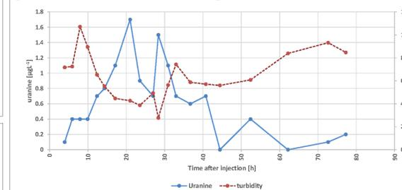
Fig. 6. Uranine concentration and turbidity in well No.4
