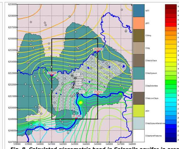
Fig. 8. Calculated piezometric head in Salaspils aquifer in area of two rivers (blue lines); observed water level in both rivers are in red color.
