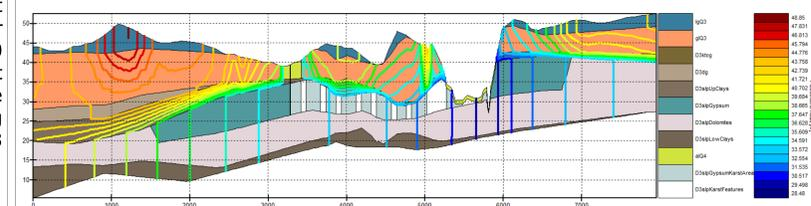
Fig. 9. Cross section of modeled area (see Fig. 7.) with piezometric heads
