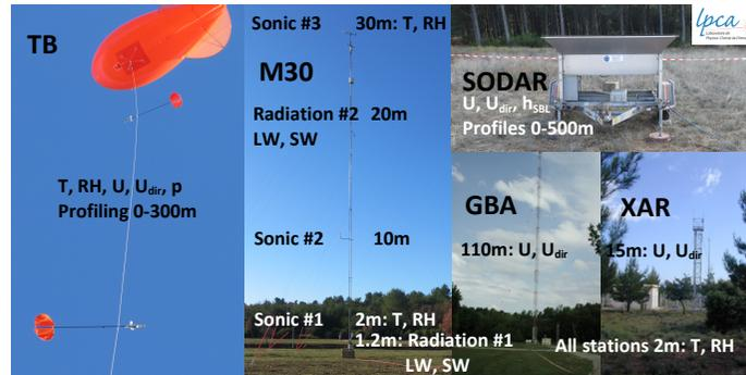
Fig.2 Sensors used during KASCADE. Height of measurements and/or profiles are given in meters (m). Radiation #1 has been measured on a separated mast at 23m distance from M30. Numbers behind sensors denotes double/triple presence implying availability of divergence observations
