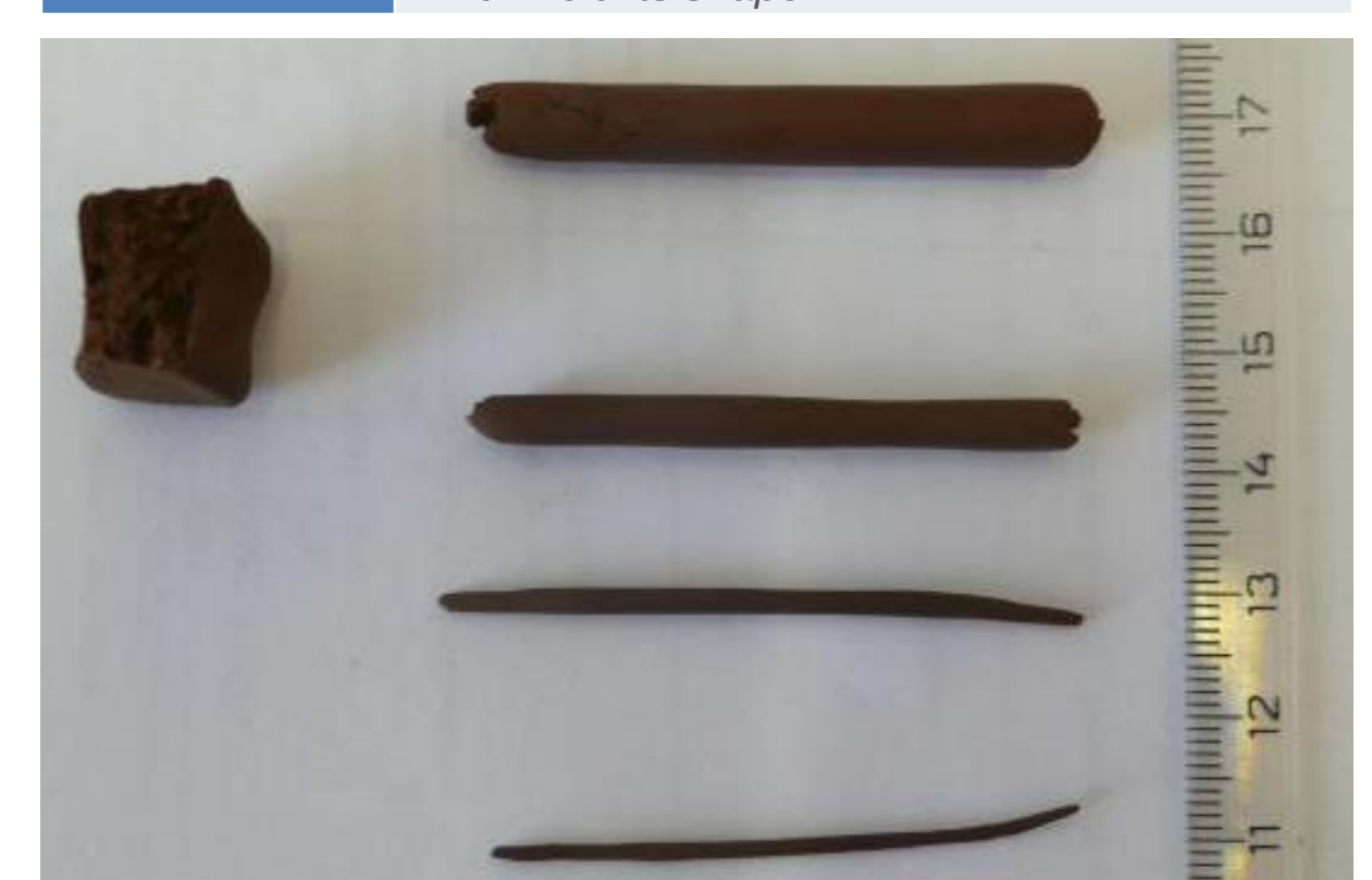
Properly prepared soil sample and wires rolled
