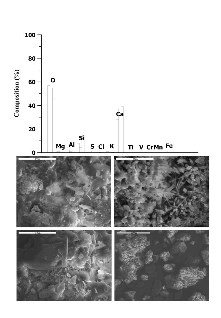
Top: Clinker elemental analysis (wt%) by SEM/EDS. um across, except for the bottom right where it is 200
