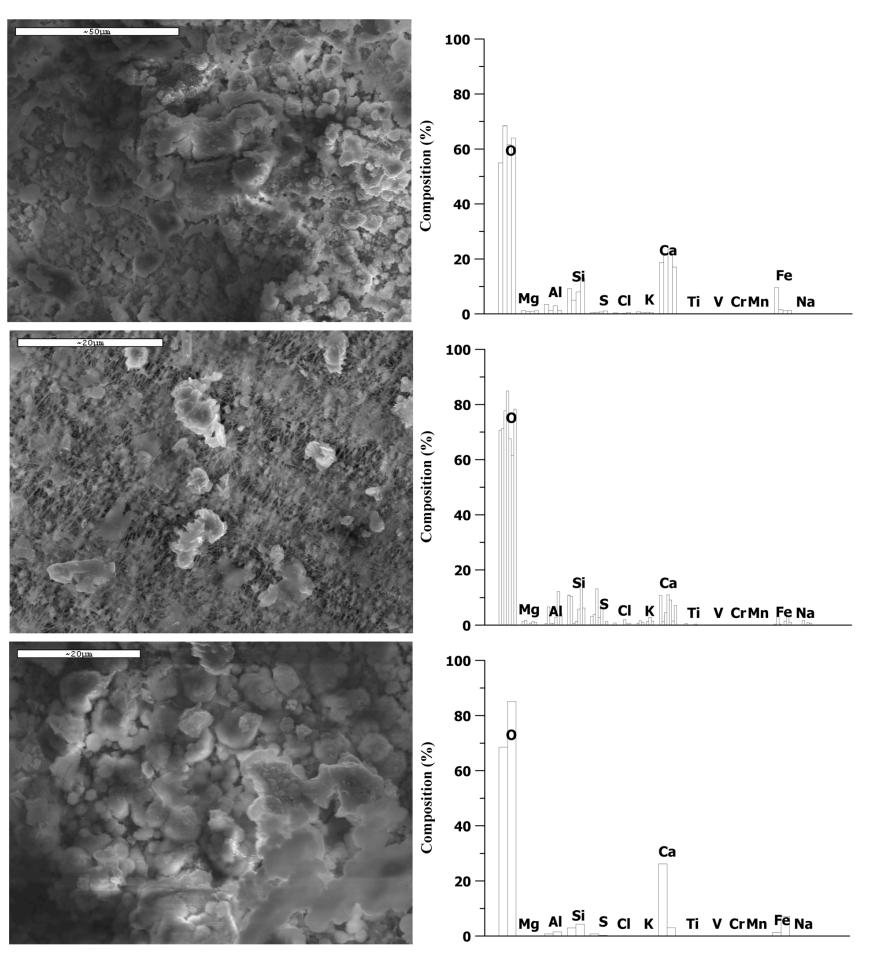
SEM micrographs of the sample (at left) and SEM/ EDS elemental analysis (wt%) results (at right) of filters (from top to bottom) No. 2 (24 June 2001), No. 4 (1
