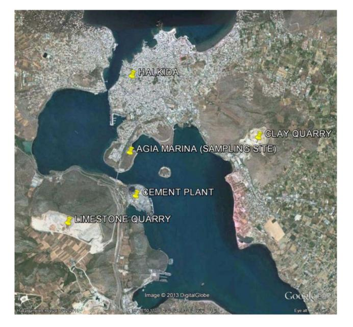
The study was conducted in the region around the town of Halkida, Greece, where the HERACLES-III cement plant (Lafarge Group) is operating (Fig), producing 2.5 Mtn of cement/yr. The production method is dry and uses pre-heating and pre-calcination. The plant operates two quarries: the limestone quarry (850,000 m2),
