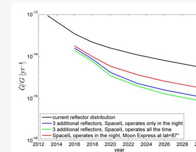
Fig. 6: Simulated accuracy for the determination of the relativistic parameter  $\dot{G}/G$ .
