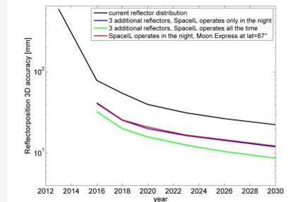
Fig. 7: Simulated 3D accuracy for the lunar reflector coordinates.
