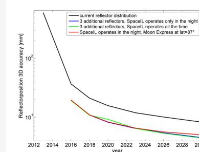
Fig. 5: Simulated 3D accuracy for the lunar reflector coordinates.
