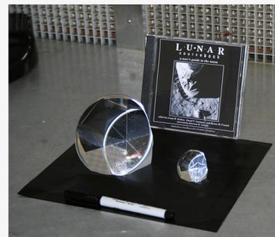
Fig. 1: Comparison of the new LLRRA-21 CCR (left) with one single Apollo-era CCR.
