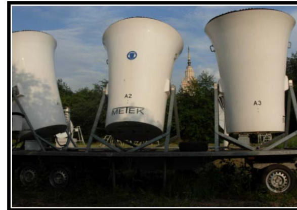
Fig.1. The “MODOS” sodar (made by METEK, Germany) at Meteorological Observatory of MSU
