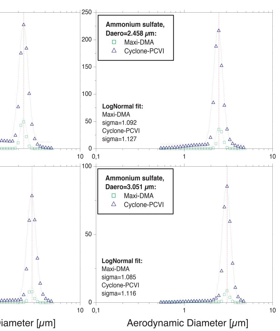
Cyclone - Maxi-DMA and the new Cyclone - PCVI combination were applied to provide quasi-monodisperse super-micron particles. Aerosol output of both setups was found to be quasi-monodisperse Application of cyclone results in a reduction of multiple charged
