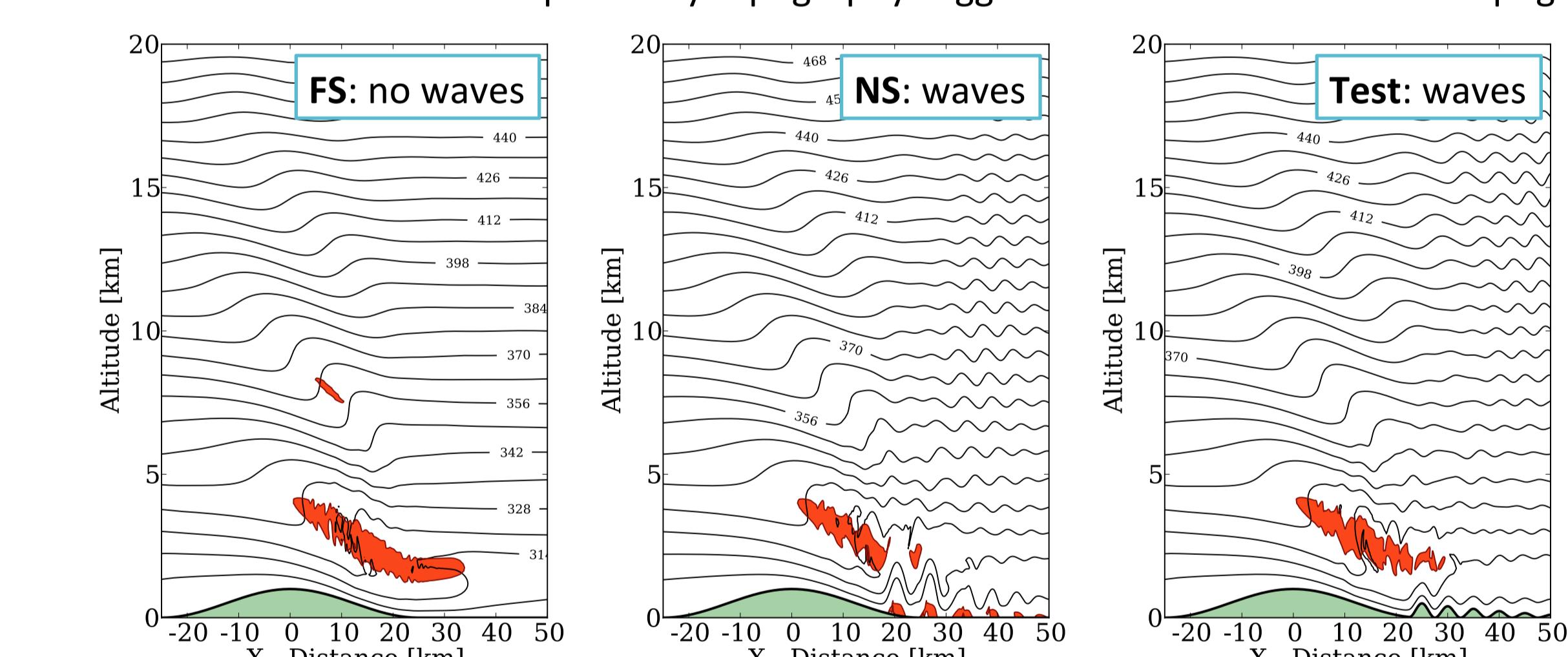
Fig. 6: Potential temperature contours of three identical simulations with the exception of the lower boundary conditions. Red contours show regions of reversed flow.
