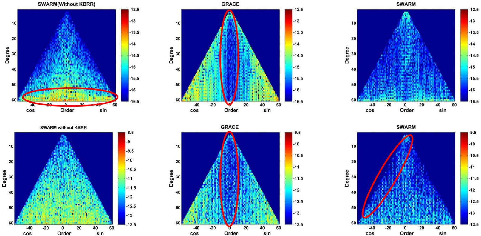
Noise free and white noise (1 cm for orbit and  $1 \times 10^{-7}$  m/s for KBRR, respectively)
