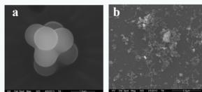
Figure 4: Secondary electron images of artefact particles within the IN/IR fraction: a) silicon oxide spheres in ISI and b) aluminium(oxide) in ICE-CVI samples.
