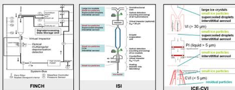
Figure 2: Sketches of the three devices (FINCH, ISI, ICE-CVI), which were used for separation of the ice nuclei/residuals.
