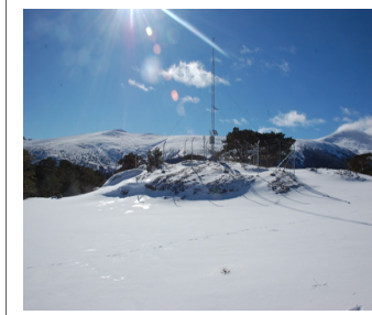
Figure 5. Seven complete stations following the WMO criteria are planned, including a four-component net radiation sensor (SNR), an ultrasonic snow height sensor (SAN), a pluviometer specialized for snow capture (PLM), air temperature and humidity sensors (THR), and wind speed/direction sensor (DVV). All instrumentation is designed to avoid the effects of icing for minimize loss of data.
