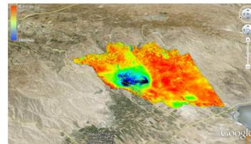
Average displacement rate [mm/year] between 2003 and 2010 with SBAS exploiting 31 Envisat ASAR acquisitions
