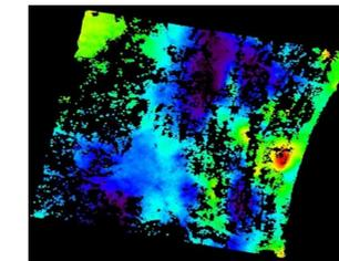
Average displacement rate [mm/year] between 2006 and 2010 with SBAS exploiting 34 Envisat ASAR acquisitions
