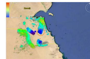
Average displacement rate [mm/year] between 2003 and 2007 with SBAS exploiting 14 Envisat ASAR acquisitions.
