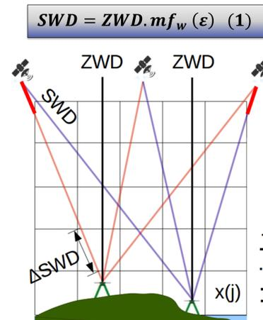
Figure 1 – GPS Tomography vertical cross section scheme.
