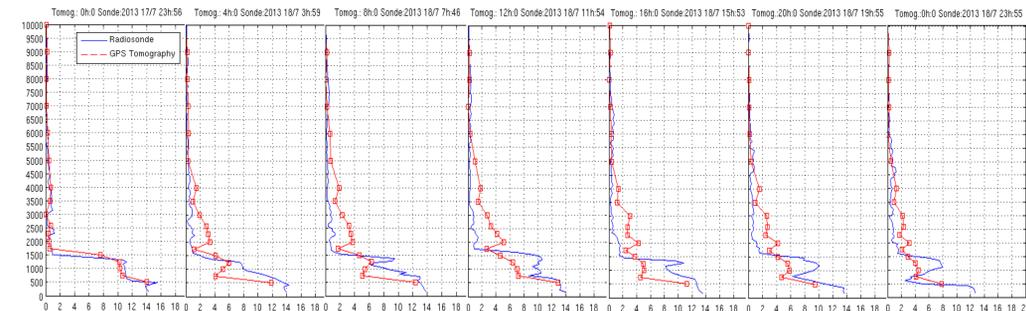
Figure 3 – Comparison between GPS tomography (x=3,y=3 column) (red), and radiosonde water vapour density (blue); 4h interval.
