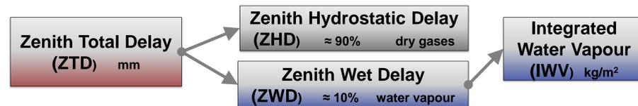
ZTD is determined from the sum of the two components, ZHD and ZWD. Usually ZHD varies very slowly in time and can be very accurately estimated using surface pressure measurements at the GPS station. ZWD is highly variable given the variability of the water vapour and the deficiencies in its observations. For this work we use the GAMIT\GLOBK software (v10.5) to process the GPS data in daily solutions.
