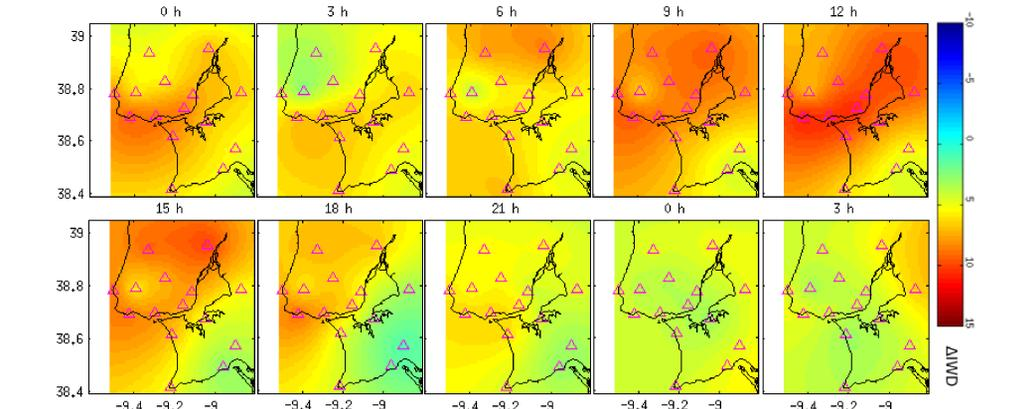
Figure 8 – 2D  $\Delta$ IWV maps from 0h July 18 to 3h July 18. Reference IWV is 0h July 17 with IWV min. to max. of 8 to 11 kg/m<sup>2</sup>
