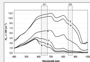
Fig.1: water spectral signature at different SSM concentrations (a: 0.013 gl-1; b: 0.023 gl-1; c: 0.062 gl-1; d: 0.355 gl-1; e: 0.651 gl-1; f: 0.985 gl-1); the two bars show the spectral position of MODIS ch1 (Red) and ch2 (Near Infrared), respectively; (adapted from Doxaran et al., 2002).
