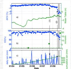
Fig.1- Green represents the water table, and blue represents the Rayleigh wave seismic velocity change of the material (Mainsant et al., 2012a)
