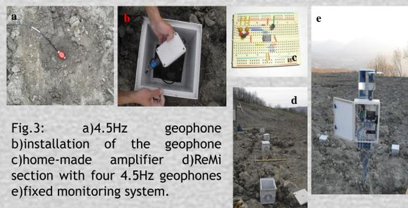
Fig.3: a) 4.5Hz geophone b) installation of the geophone c) home-made amplifier d) ReMi section with four 4.5Hz geophones e) fixed monitoring system.
