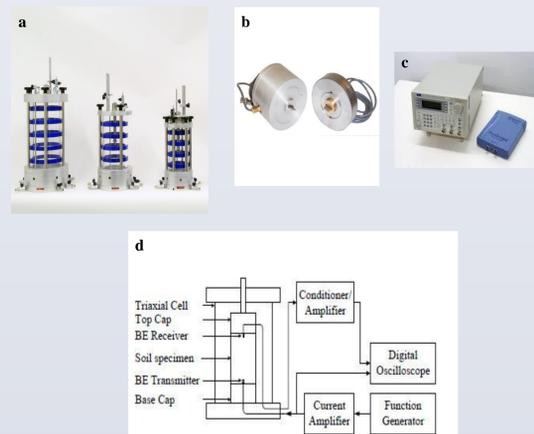
Fig.4: a) modified triaxial cell, b) bender elements, c) signal generator and digital oscilloscopy, d) simple scheme of the lab test.
