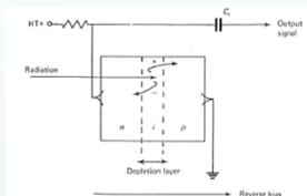
Fig 1 The PiN diode as a radiation detector (Tait, 1980)
