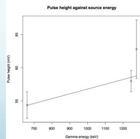
Fig 5 Median pulse heights against source energy. An average <sup>60</sup>Co energy of 1.25 MeV has been assumed, and the 0.511 MeV contribution from <sup>22</sup>Na ignored. Error bars are two standard errors.
