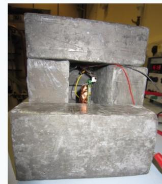
Fig 6 Testing in lead castle to exclude background gamma radiation
