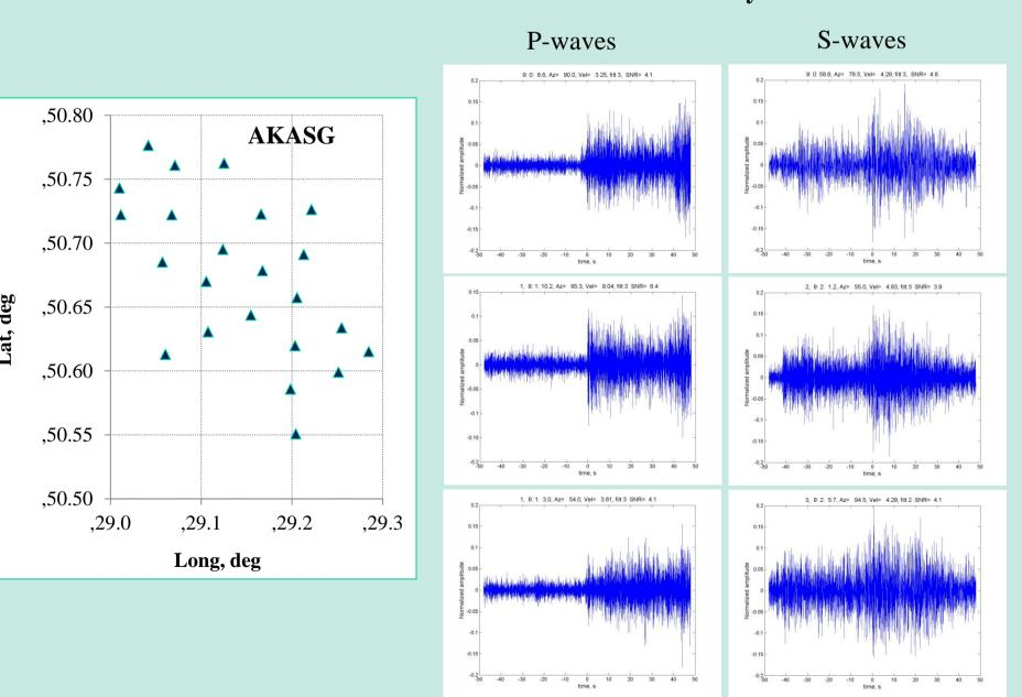
Station AKASG includes 23 vertical channels and has aperture of 25 km. All events were detected by standard STA/LTA procedure for those days where continuous data was available. We present several typical waveforms (detection beams) for P- and S-wave arrivals. Overall, these signals are similar to those at MHVAR and can be used for joint analysis – association of detections into events.
