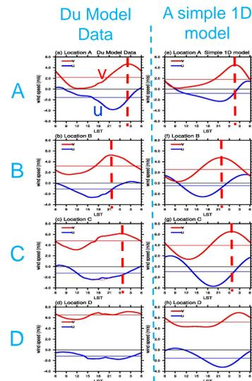
Fig.2 Diurnal variations of mean 950-hPa local u- and v- wind component at locations A, B, C and D from the Du Model Data (a-d) and the simple 1-D model (e-g) with mean values indicated by the thin solid lines
