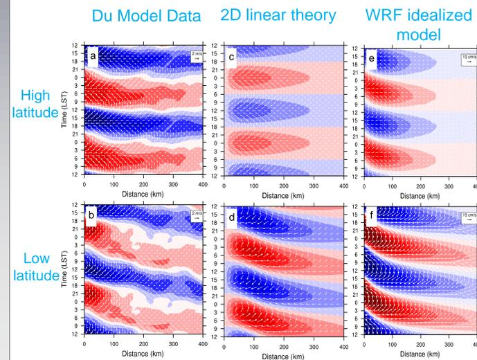
Fig.4 Longitude-time Hovmöller diagrams of perturbation horizontal wind vectors and vertical velocity at 950 hPa averaged (shaded; m s<sup>-1</sup>) over the a) northern and b) southern boxes in Fig. 1b from the Du Model Data; the present linear solutions at c) 35N and d) 25N; idealized WRF experiments with terrain and surface heating at latitudes e) 35N and f) 25N.
