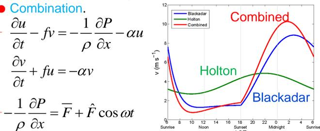
Fig.3 Comparison of the diurnal variations of among the Holton mechanism (green), the Blackadar mechanism (blue) and their combination (red)
