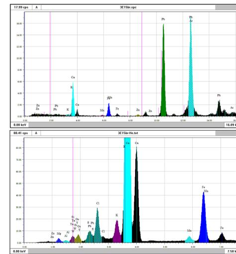
Figure 5 | XRF spectrums of a sample from a sculpture in East Portal, at high and low X-ray energy, respectively.
