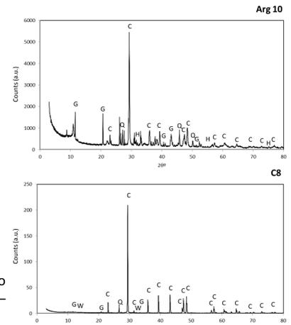
Figure 4 | XRD patterns of two samples (C – calcite, Q – quartz, G – gypsum, H – halite, W – weddellite).
