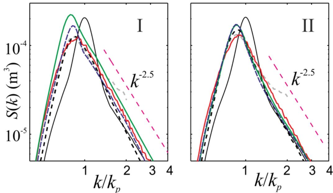
Evolution (first 150 periods) of spectrum I (narrow in angle) and II (wider in angle), with a direct comparison of 5 approaches (modified from figure 7a,b of Xiao et al 2013)
