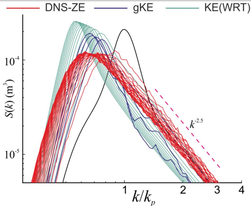
Long-term spectral evolution for spectrum I, with the comparison of DNS-ZE and both kinetic equations (KE and gKE). Spectra are plotted every 300 periods
