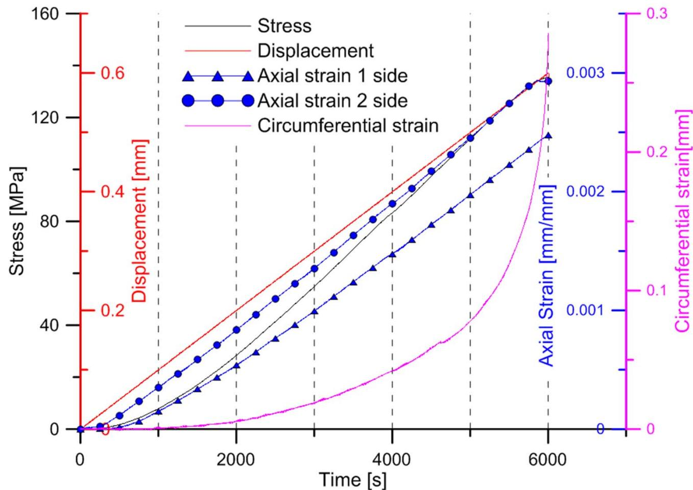
Loading with constant strain rate 0.006 mm/min
