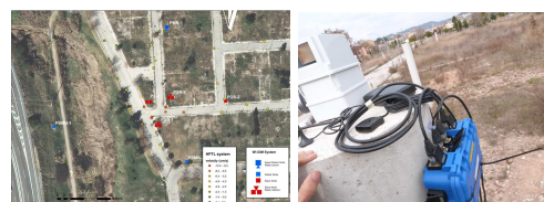
Figure 5 (up) Different components that compose the WI-GIM sensors: Radar device, decawave (radio sensor), master/slave node box, battery, communication modem (for master nodes) and GPS antenna (optional). (above, left) WI-GIM system distribution for Sallent site. (above, right) WI-GIM sensors installed in Sallent test site.
