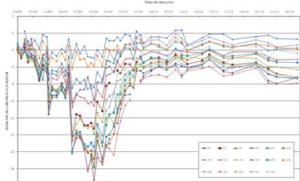
Figure 2 (up) Subsidence velocities of the closest points to the area of maximum subsidence, from March 2008 to May 2014. Figure 3 (left). Distribution in plant of subsidence (IGC,2008).
