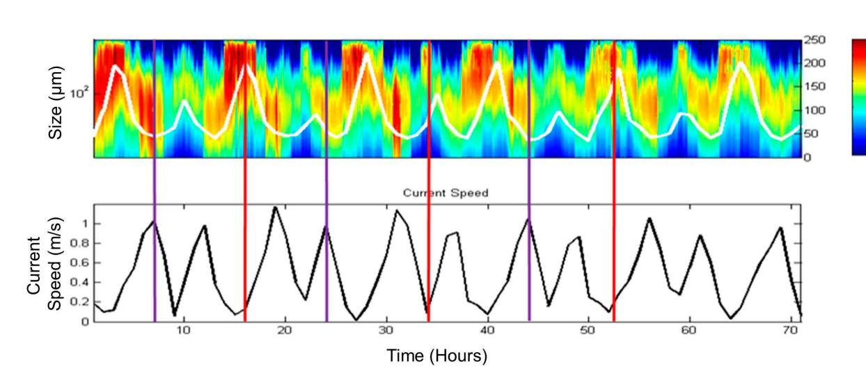
The data above was recorded by a Sequoia Scientific LISST-100X Type C in the Dee Estuary during February-March 2009, with current speeds in the bottom panel provided by an ADCP.
