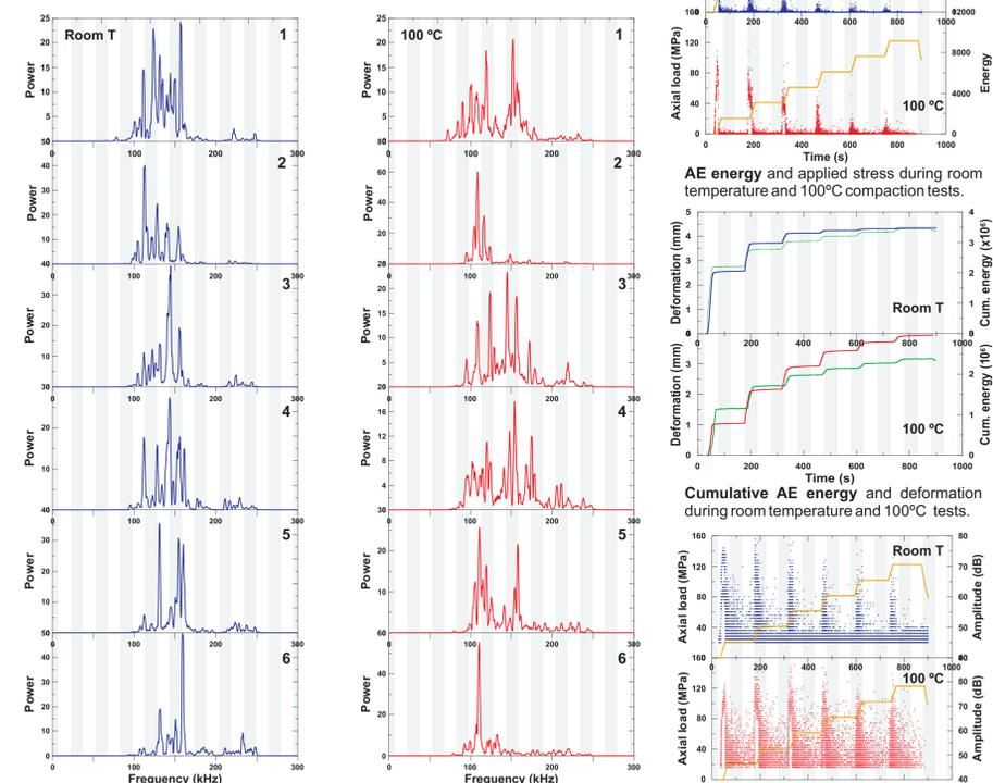
Power vs frequency graphs for each of the six stages of the testing process. Fast Fourier Transformations were used to transform waveforms from the time to the frequency domain, both for room temperature (left) and 100°C (right).
