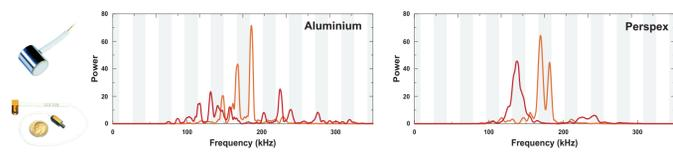
Power vs frequency tests performed with the Micro200HF (dark brown) and HD50 (light brown) sensors. To test the quality of the sensors, a pencil lead with a 0,5 mm diameter and a 2H hardness was broken by pressing against an aluminium (left) and perspex (right) surface to simulate acoustic emission.
