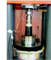
Tests were carried out in servocontrolled hydraulic press and PCD2K multi-channel controlling system. PAC Micro200HF and HD50 AE Sensors were attached to the compression device.
