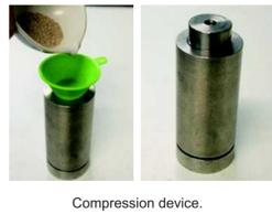
Silica sand was used in this study. Its grain size distribution curve is shown in the left figure. The sample was compacted in a cylindrical compression container made of stainless steel with an outside diameter of 55 mm and an inside diameter of 35 mm. In compression tests, the total height of the sample in the container was 10 mm, equivalent to about 13 g.
