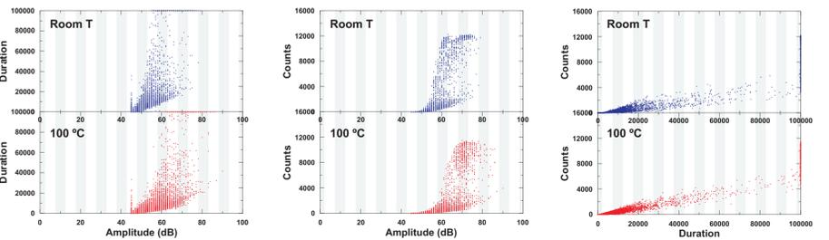
Duration vs amplitude, counts vs amplitude and counts vs duration crossplots of AE signals detected during the testing. The upper graphs show the results for room temperature, while the lower figures show those for 100°C.
