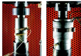
Experimental setup showing AE sensors attached to the compression device prepared for the test.
