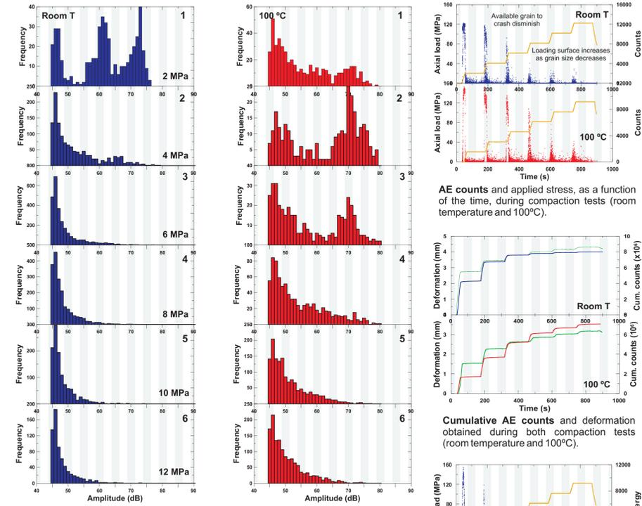
Amplitude distribution histograms of all the events generated during each of the six stages of the testing process, both for room temperature (left) and 100°C (right).
