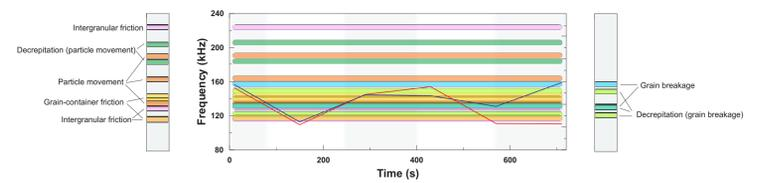
Main frequencies for each stage of high-pressure compression tests are shown using blue (room temperature) and red (100°C) lines.
