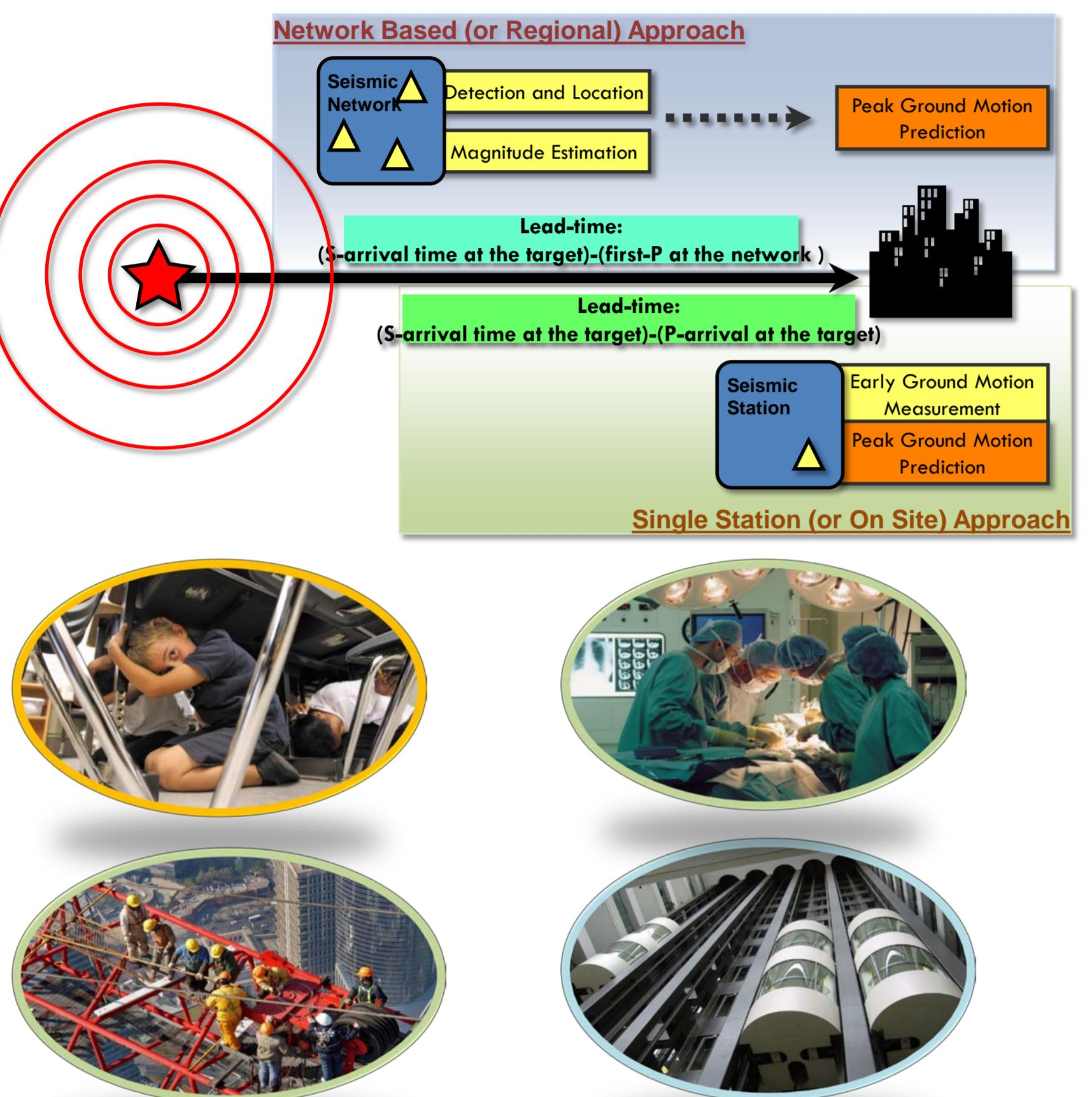
Earthquake early warning systems (EEWS) are Real-time, modern information systems that are able to provide rapid notification of the potential damaging effects of an ongoing earthquake, through the fast telemetry and processing of data from dense instrument arrays deployed in the source region of the event of concern (regional EEWS) or surrounding the target infrastructure (site-specific EEWS).
