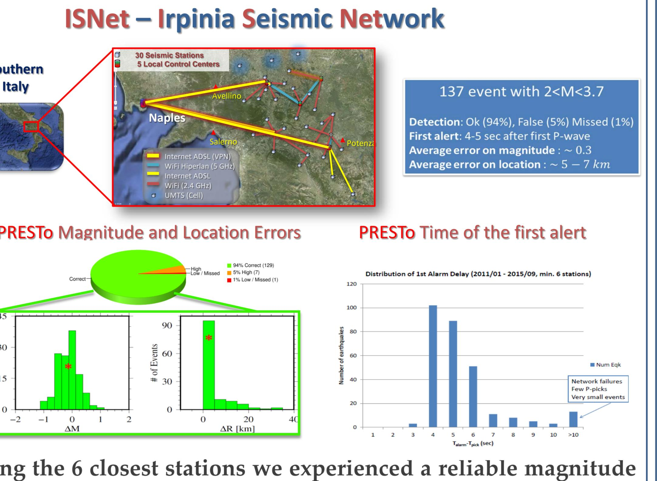
Using the 6 closest stations we experienced a reliable magnitude estimation in 94% of cases and a hypocentral location error smaller than 5 km in 76% of cases. The time of the first alert is 4-5 seconds on average, including computation and telemetry delays.
