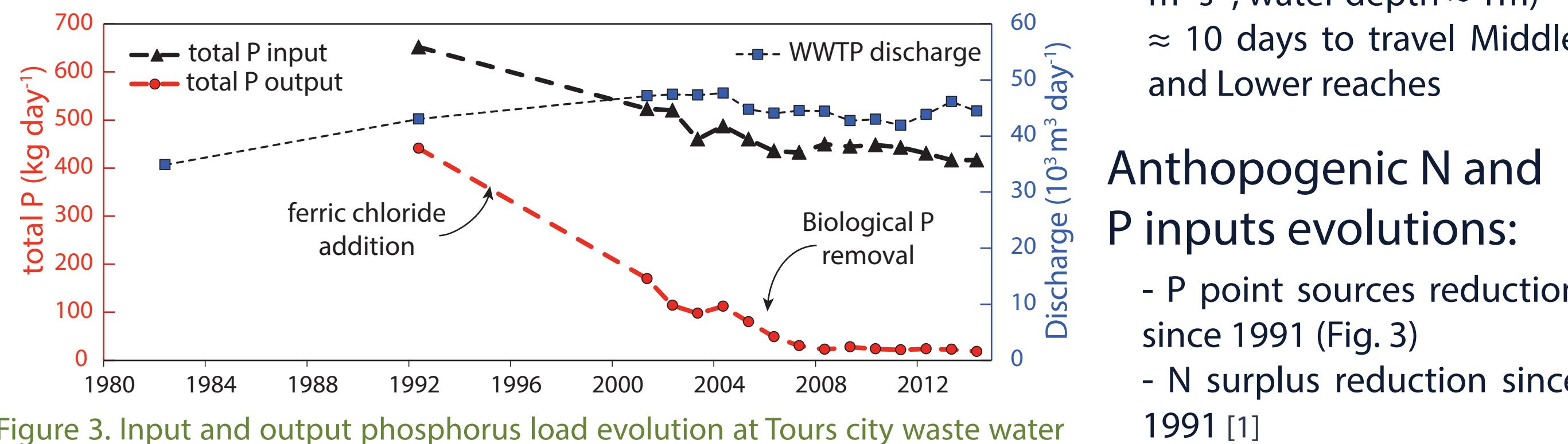
Figure 3. Input and output phosphorus load evolution at Tours city waste water treatment plant (400 000 inhabitants equivalent)
