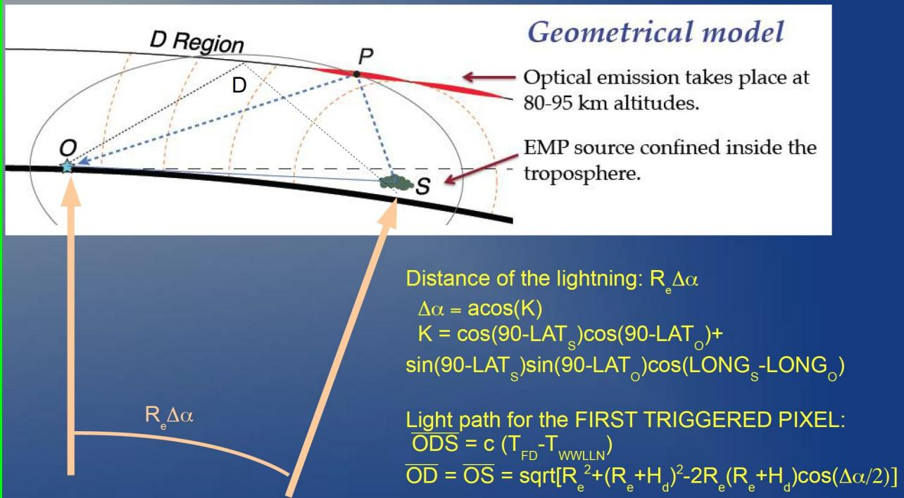
Photons detected by the FD camera are corrected for distance from the base of ionosphere (assumed at 85 km ), and for the surface observed by each pixel.
