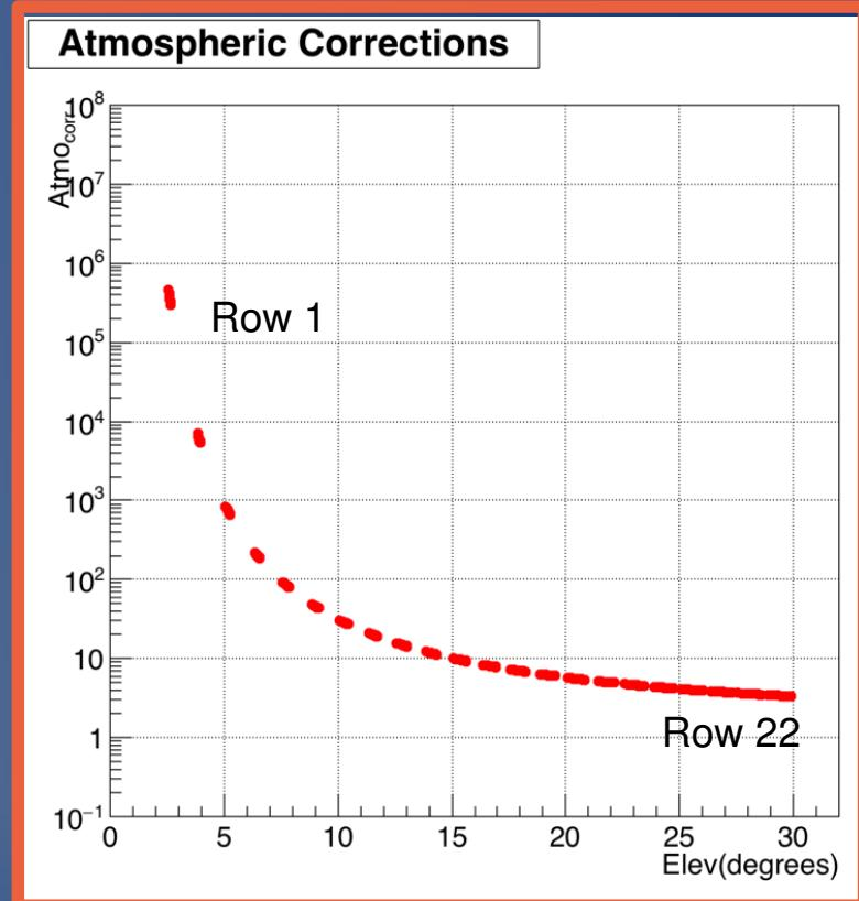
Photons detected by the FD camera are corrected for distance from the base of ionosphere (assumed at 85 km), and for the surface observed by each pixel.
