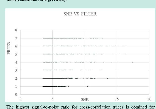
filters 4 to 6. The performance of the low-frequency filter (1-3 Hz) is likely affected by the high-level ambient noise near 1 Hz. However, this filter is important for Rg-wave, which is most sensitive to the position of source within the quarry. This filter was successfully used to distinguish quarry 19 from adjacent quarries.
