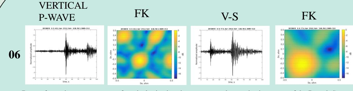
Beams for various components of vertical seismic sub-group steered towards the source of the P- and S- wave from quarry 06.
