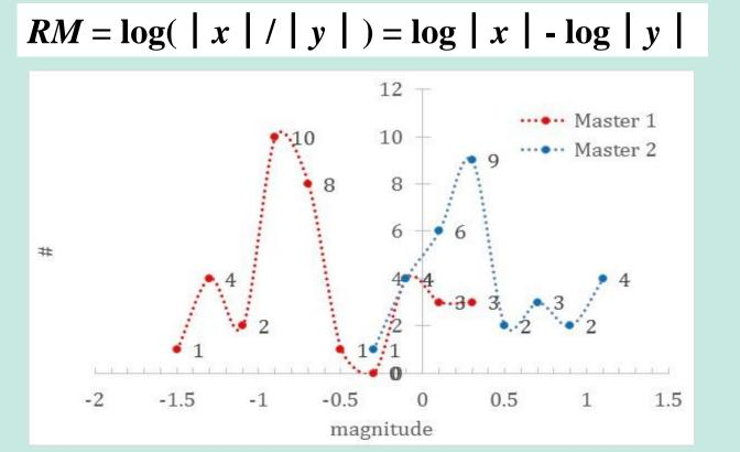
For events with correlating signals, one can define relative magnitude. The distribution of relative magnitudes for two masters demonstrates that master 1 is likely larger than master 2. For master 1, other blasts were generally smaller (negative RM), and master 2 was slightly smaller than other events from the same quarry.
