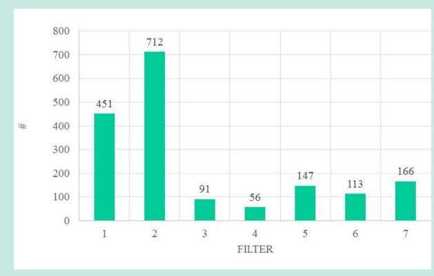
The importance of various filters for cross correlation is demonstrated by the frequency distribution of filters actually detected signals from the same source. The best filter depends of the properties of generated signal as well as ambient noise conditions for a given day.
