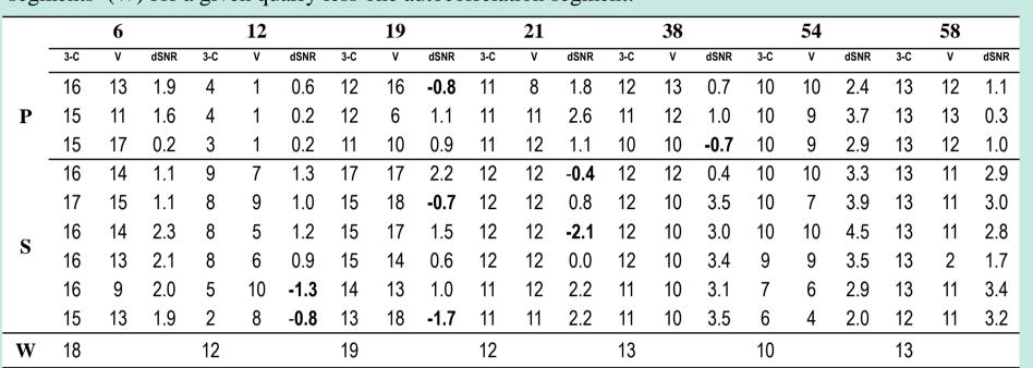
Results of  $SNR_{CC}$  calculations for 13 segments from quarry 21 with templates for quarries 12 (21/12), 19 (21/19) и 21 (21/21). Averaged values are listed.
