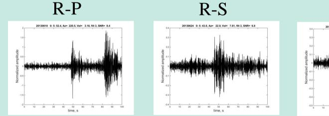
Beams for two components (R and T) of the 3-C group steered towards the P- and S-wave sources of quarry 06. Peak SNR value for three beams can be observed at transversal (T) as well as at radial (R)components.. There is a P-wave arrival from quarry 6 observed on the beams of vertical channels despite the corresponding traces are steered towards the source of S-wave.
