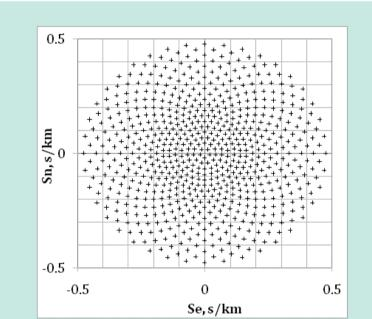
Standard slowness set  $(S_e, S_n)$  for automatic beamforming. Sn and Se are in the range -0.5 s/km to +0.5 s/km. Azimuth resolution better than 4.5°.
