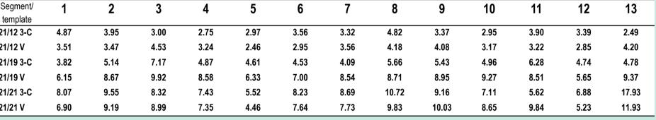
The number of detections by 40 waveform templates after cross correlation with OWN and OTHER segments (total 104 segments) before and after application of slowness threshold of 0.05 s/km.
