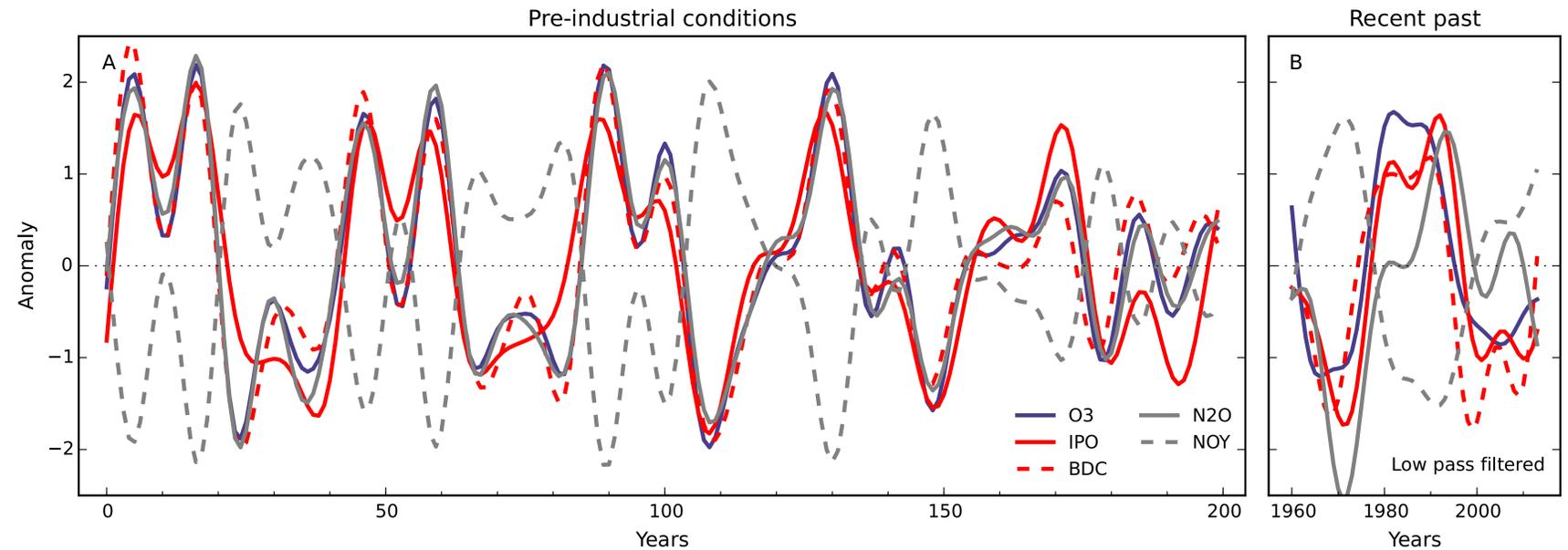
A long simulation including only internally generated variability (A) and a simulation of the recent past (B) show that the IPO is associated with the general circulation in the stratosphere - the Brewer-Dobson circulation (BDC). Changes in the BDC modulate ozone loss in the tropical middle stratosphere via NO<sub>y</sub> chemistry.
