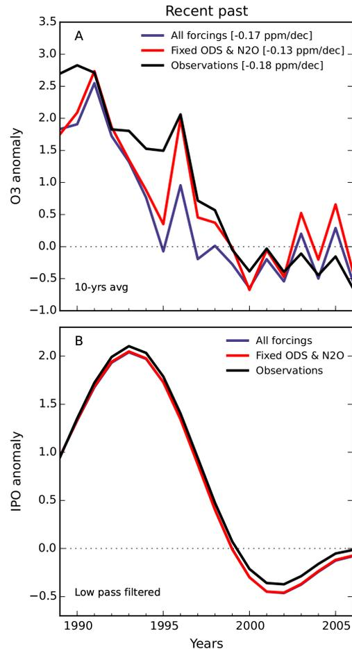
Simulated mid-stratospheric tropical ozone anomalies show a sharp decrease for the 1990-2000 period and persistently low levels since ~2000 (A), which is in very good agreement with observations and largely unrelated to forced signals (i.e. ozone depleting substances and N<sub>2</sub>O emissions).
