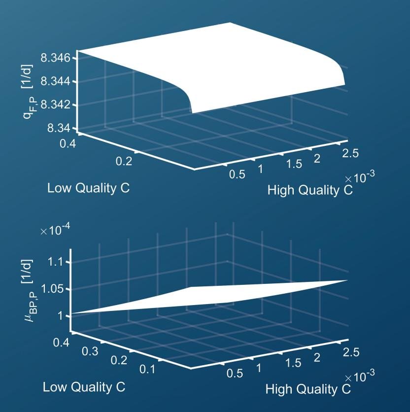
Examples of kinetic functions that define characteristic time scales for the pesticide variable. Cometabolic degradation  $q_{F,P}$  is the dominant process.
