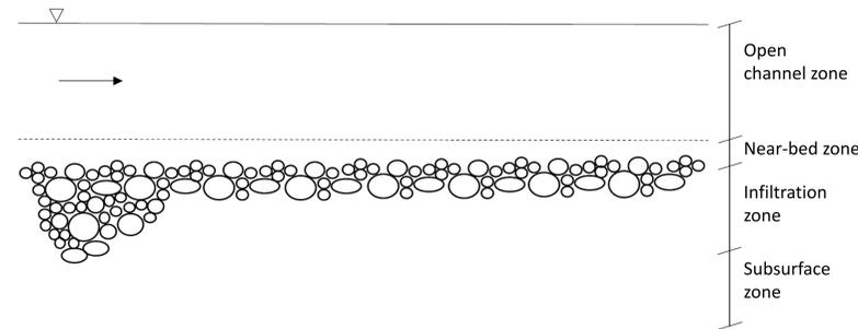
Figure 2: The four different zones within the depth profile of a river
