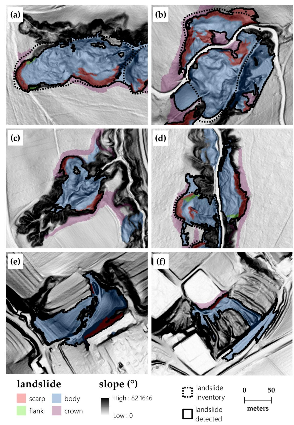
a-b: detected landslides in inventory. c-d: detected landslides outside of inventory. e-f: false-positive classification due to similar morphometric characteristics.
