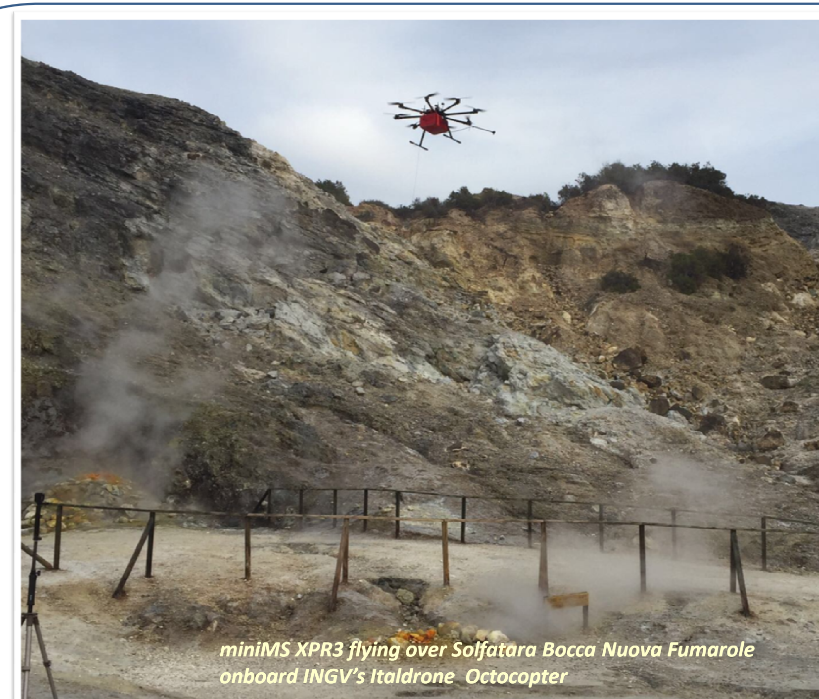
miniGAS NTX integrated to Italdrone Octocopter at Solfatara 2016 Deployment
