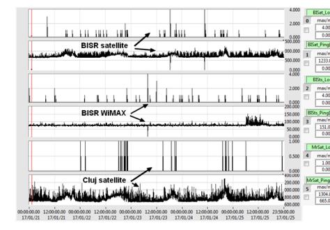
Fig. 14 Satellite EUTELSAT and WiMAX land communication latency
