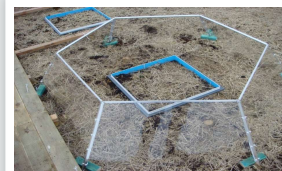
Figure 5: Selected plots were equipped with Open-Top Chambers (Molau and Mølgaard, 1996): UV resistant polycarbonate (3 mm): 2.08 m lower diameter, 1.50 m upper diameter, 0.6 m height.
