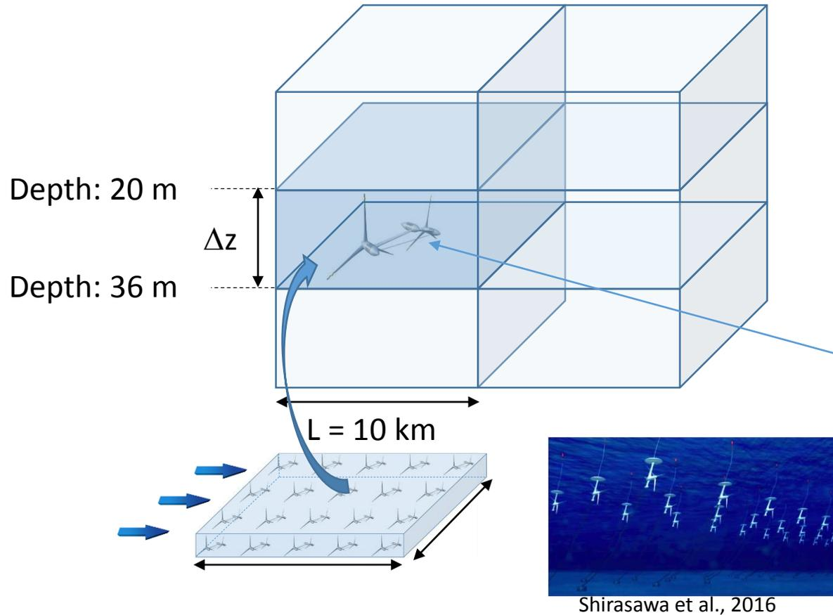
**Virtual EPU**s are represented by a **Quadratic Drag Force** added to the model momentum equation **at the location (lon, lat, depth)** that the EPU is assumed to occupy.
