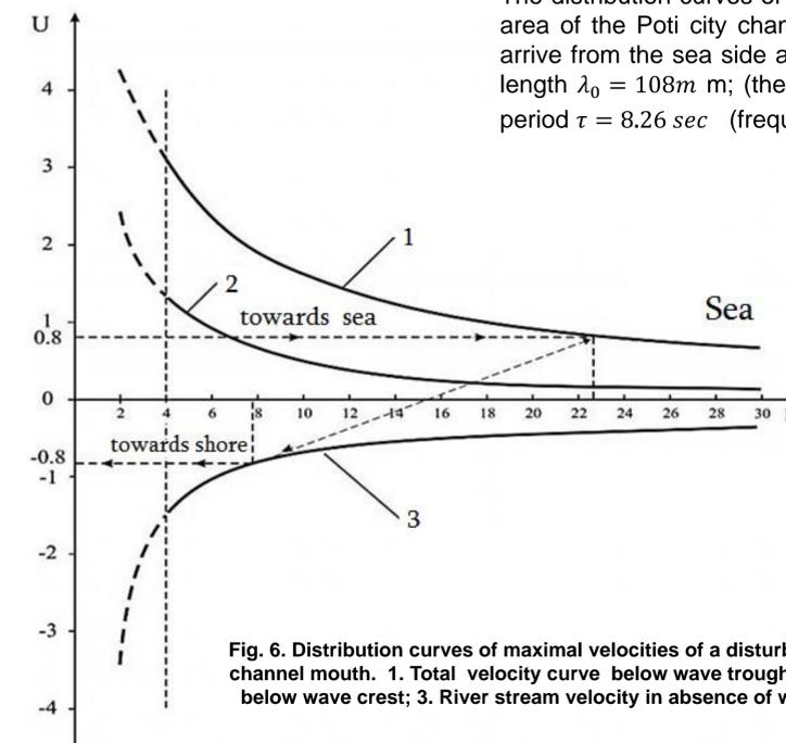
Fig. 6. Distribution curves of maximal velocities of a disturbed stream near the city channel mouth. 1. Total velocity curve below wave trough; 2. Total velocity curve below wave crest; 3. River stream velocity in absence of waves to the Poti coast
