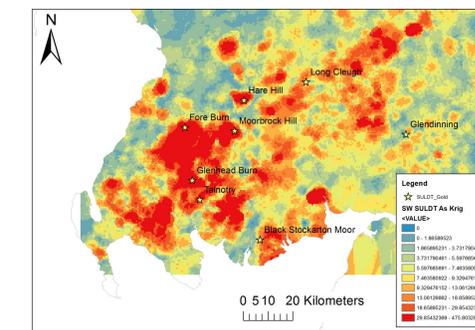
Figure 5: Interpolated map of arsenic in stream sediments in SW Scotland. BGS Licence 2015/063GC ED. ©NERC.
