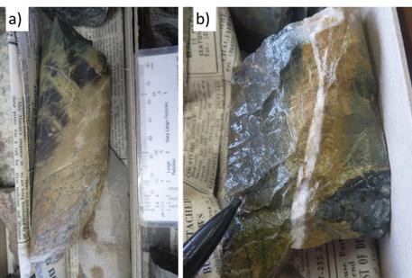
Figure 2: Examples of hydrothermal alteration and veining around porphyritic granodiorite intrusions in drill core from Black Stockarton Moor; a) sericitised greywacke immediately above a granodiorite contact @221 m in BH7; b) sericite halo around quartz vein above granodiorite sheet @193 m in BH7.
