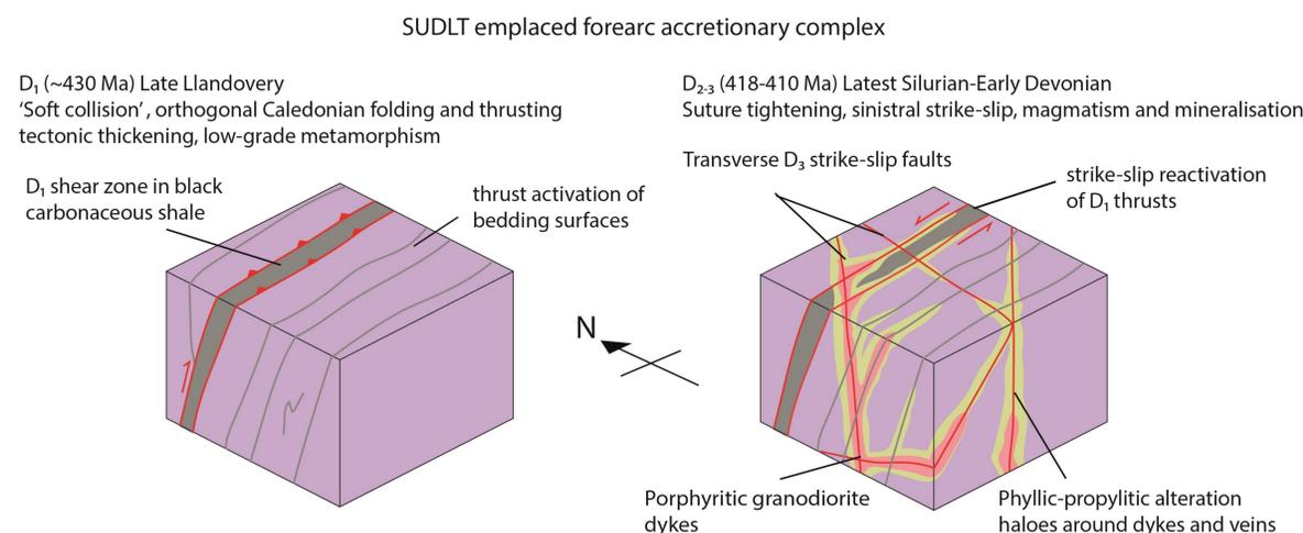
Figure 4: Schematic block models illustrating the structural and metallogenic development of the SUDLT.
