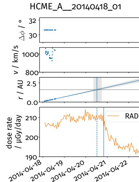
Figure 1: Example of an ICME observation at STEREO-HI combined with MSL/RAD Forbush decrease
