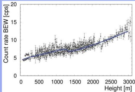
A **new model** accounting for the presence of **atmospheric <sup>222</sup>Rn** provides a good reconstruction of the BEW count rate vertical profile, showing the **potential of offshore AGRS measurements in <sup>222</sup>Rn monitoring**
