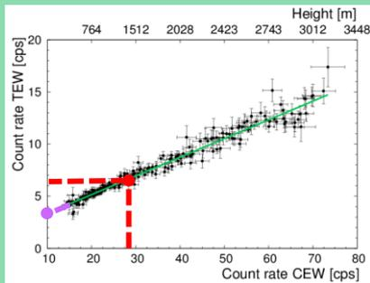
Count rates **linear regression lines** allow for discriminating **cosmic** from **experimental setup radioactivity** background, assessing **background count rates** during AGRS regional surveys and determining **Minimum Detectable Abundances**
