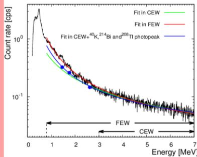
The **cosmic spectral shape** of a measured gamma spectrum was reconstructed by using as additional constraints to the high energy tail the cosmic count rates measured in the <sup>40</sup>K, <sup>214</sup>Bi and <sup>208</sup>Tl photopeaks
