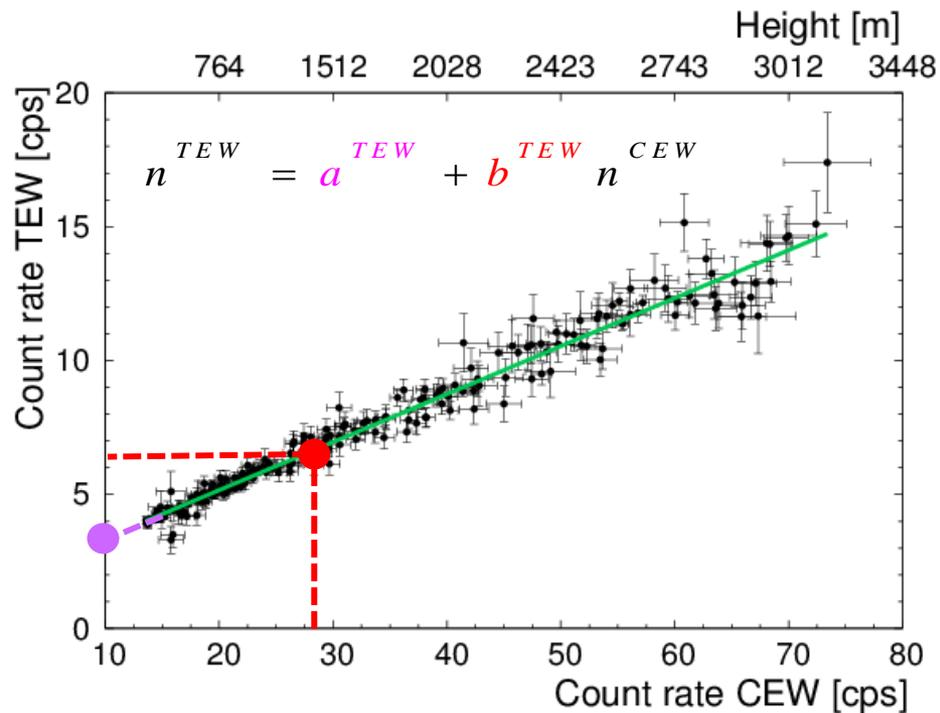
Linear regressions between count rates in the *i*-th energy window and in CEW allow for correcting for background the CRs measured during regional AGRS surveys
