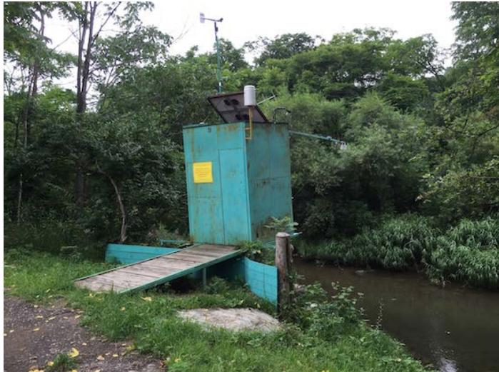
Automatic device for water level measurements with high temporal resolution at the place of rare water discharge measurements
