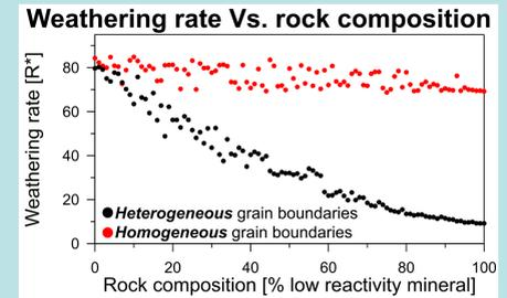
The grain boundary reactivity determines whether mechanical detachment is the dominant mode of weathering.
