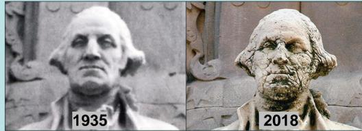
In micrometer grained rocks, enhanced dissolution at grain boundaries cause mechanical detachment of particles.
