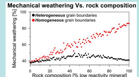
The number of detachment events in the different models reflects the transition from the detachment of tiny sub-grains to the detachment of large complete grains.
