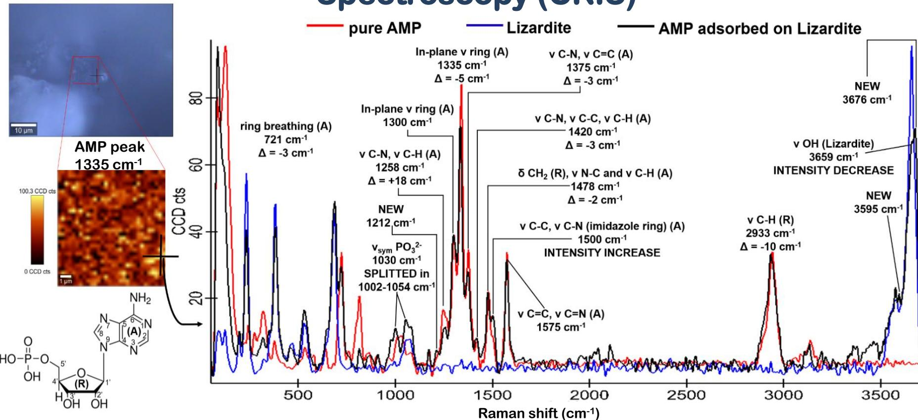
Splitting of phosphate stretching vibration, decrease of intensity for stretching of lizardite hydroxyl group, and appearance of new bands in the phosphate and hydroxyl stretching regions, indicate that **AMP molecules interact mainly through the phosphate group**, presumably forming covalent bonds with metal-hydroxyls of lizardite
