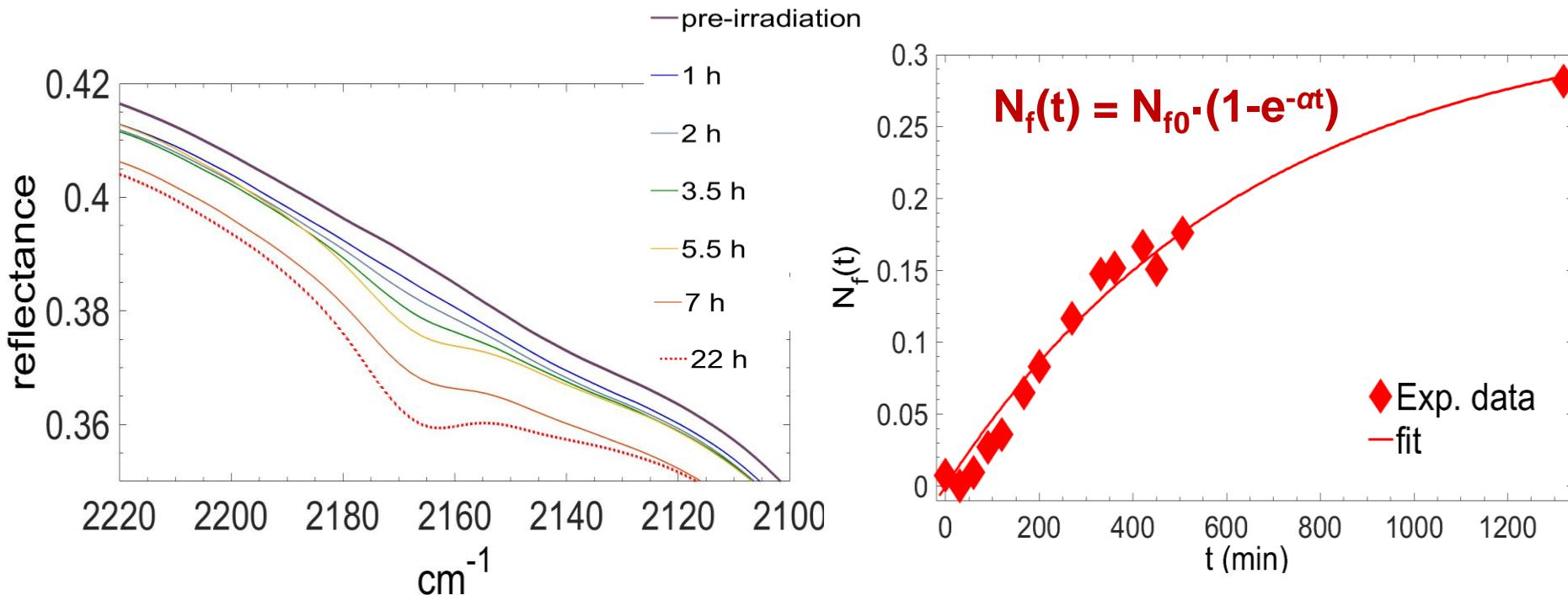
**Formation of a new peak at  $2164\text{ cm}^{-1}$ , likely corresponding to a cyanate OCN- fragment ( $\sigma_f \approx 10^{-22}\text{ cm}^2$ )**
