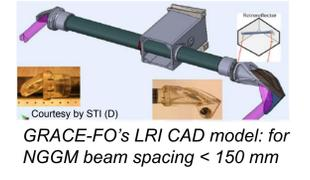
GRACE-FO's LRI CAD model: for NGGM beam spacing < 150 mm
