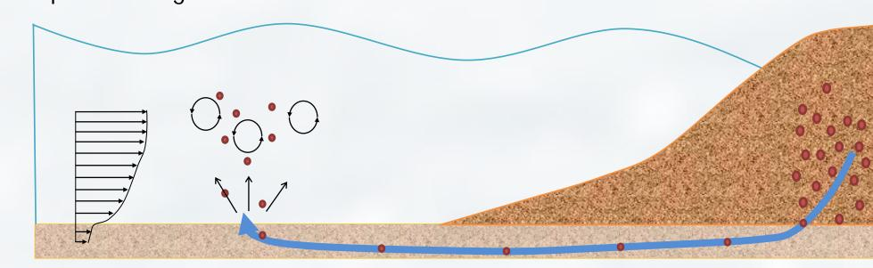
First results show, that for a planar seabed the vertical transport is dominated by the diffusion velocity, whereas the horizontal transport is governed by the wave motion. The mixing however occurred in the porous media itself while the spatial transport of the tracer takes place in the water column.
