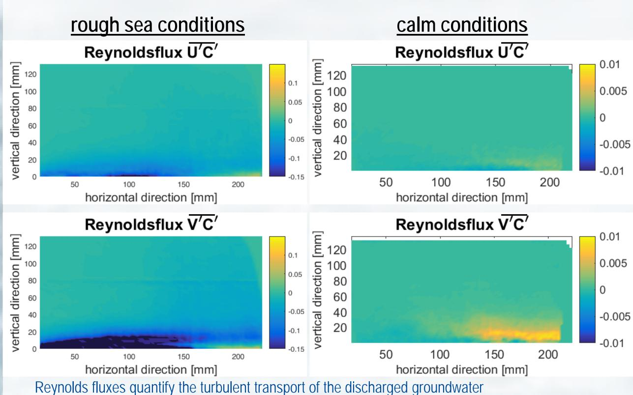
The fluxes reveal the interaction between wave action, turbulence and scalar transport in the shallow coastal zone. The cross correlation between the horizontal velocity and the concentration fluctuations constitutes the Reynoldsflux  $\overline{u'c'}$ . It indicates the horizontal turbulent transport, whereas  $\overline{v'c'}$  indicates the vertical transport. Here, the turbulent vertical transport fluxes are always dominating over the horizontal fluxes
