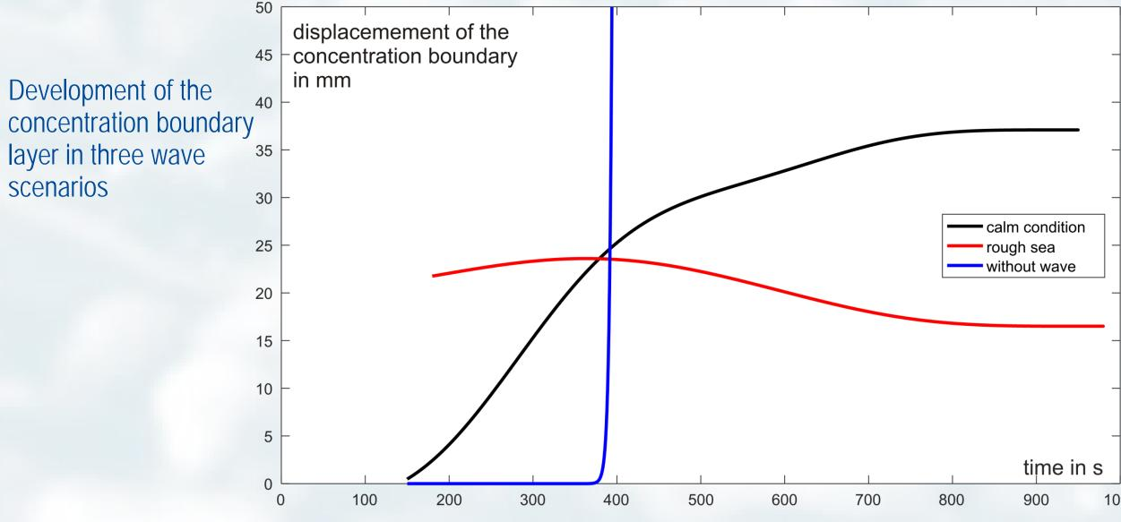
The rough sea scenario (max.velocity:2m/s, period: 3.3s) showed a very fast distribution of the tracer out of the ground into the water column. On the contrary the calm wave scenario (max.velocity:0.5m/s, period: 2s) shows a slow and continuous layering of the tracer above the ground. To compare those results the outflow of tracer without wave action is plotted.
