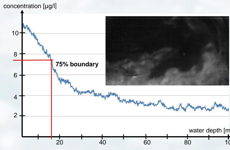
For the quantification of the distribution, a 75% boundary determined. This boundary was observed during a time period of 15 minutes. For the first experiments two different wave scenarios were produced.
