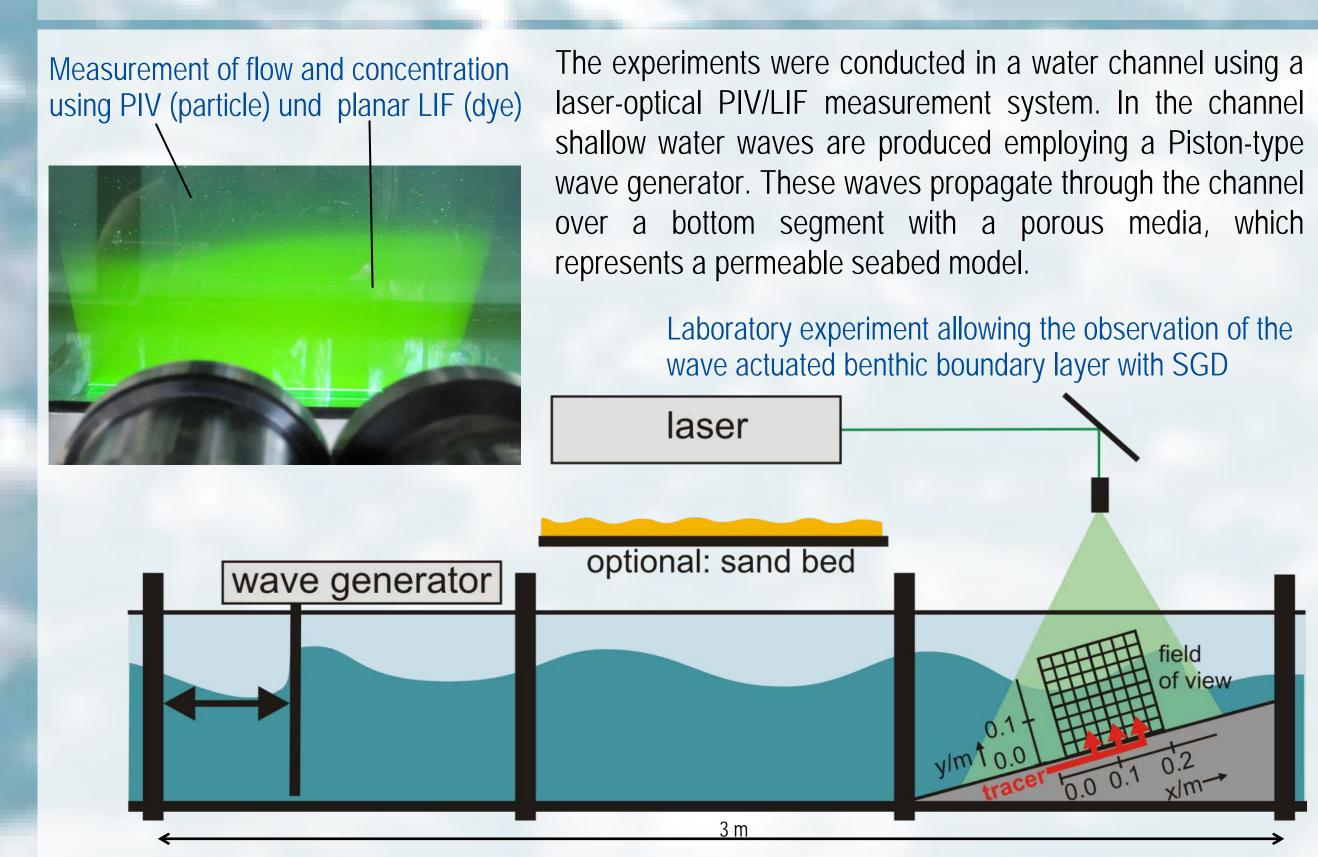
Through the seabed model a fluorescent tracer is injected which then can be detected by the laserinduced-fluorescence method (LIF) and allows a quantitative measurement of the tracer volume flow into the water column. Simultaneously images obtained by particle image velocimetry (PIV) provide instantaneous velocity fields of the unsteady mixing flow.
