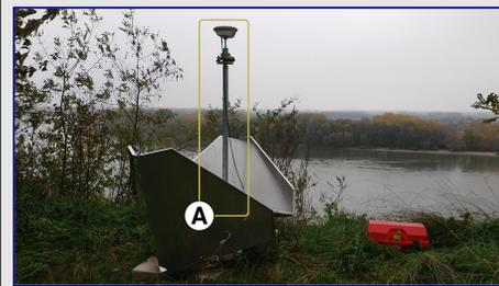
Figure 3: Reflector IB2 with rod and GNSS antenna (A); rod and antenna are only present during GNSS observations
