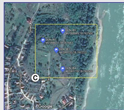
Figure 5: Spatial distribution of reflectors with the landslide area outlined (C); from Google Maps
