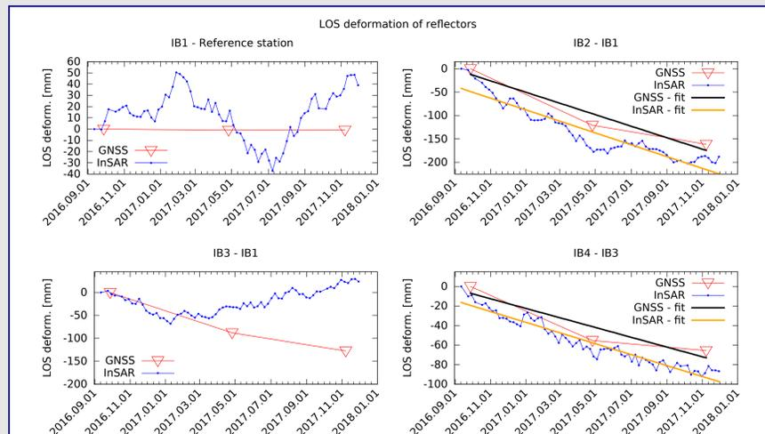
Figure 6: LOS deformations derived from InSAR and GNSS measurements at reflector IB2 with respect to (w.r.t) IB1, IB3 w.r.t IB1 and IB4 w.r.t IB3 and fitted linear trend. The InSAR signal at IB1 is most likely due to atmospheric effects. Negative LOS deformation means movement away from the satellite.
